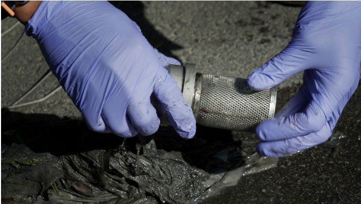
A crew retrieves a probe for testing on the West Side of Chicago. The stainless steel canister has a mesh surface so liquid flows in.
