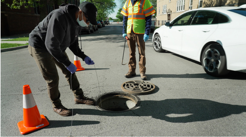
A crew retrieves a probe for testing on the West Side of Chicago. The stainless steel canister has a mesh surface so liquid flows in.
